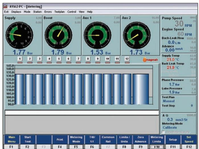
Figure 2 AVM2-PC metering screen display
