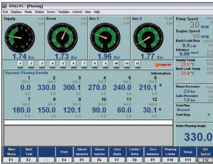
Figure 3 AVM2-PC phasing screen display
